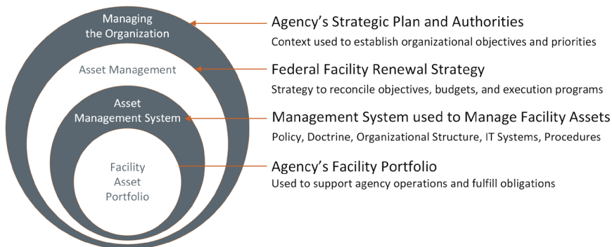
FIGURE 3-1 Relationship of key terms relating a facility asset management system to an asset management system, based on ISO 55000.
